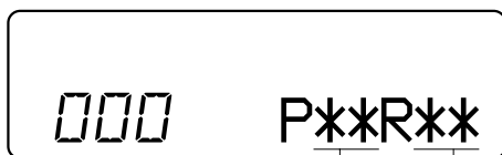
Total count of play system errors (hex.) Total count of record system errors (hex.)
